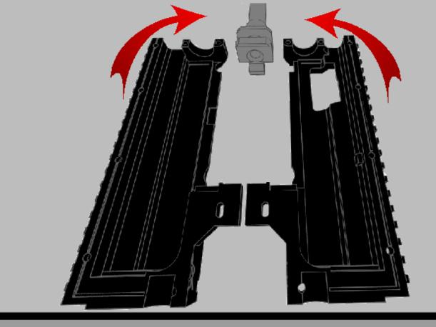
Now it's time to start to assemble the upper receiver! but don't worry, it's easier than all those screws make it out to be. You can lay both halves flat on a table with the barrel in between them and clap them together with the front sandwiched between them.
